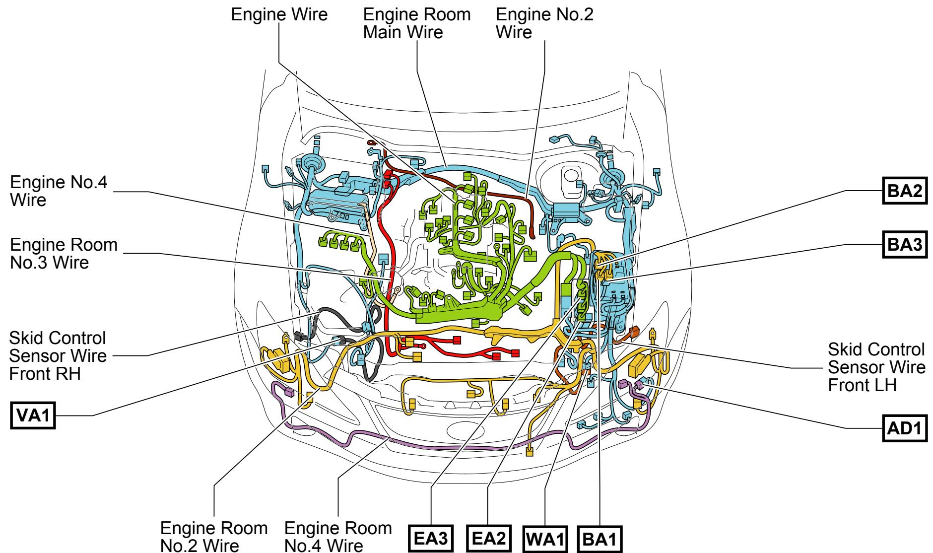
Wire and Wire in Engine Compartment <LHD 2AD-FHV, 2AD-FTV>
